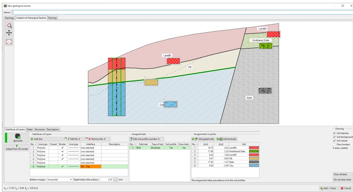
We will also adjust the landfill interface. This time, we will delete the old interface and create a new one. This procedure is simpler, but we will lose the information about the original shape. In this case, after deleting the interface, we will also need to extend the line, which creates the fault so that the areas are closed.
